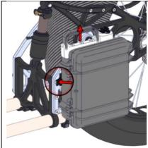
ii. While pressing down on the selflocking tab, grab the handle mounted on the top of the battery case and pull upwards.
