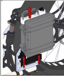
iii. Once the case begins to move along the case slots it is no longer necessary to manually engage the tab. The battery will slide up and out of the slots.
