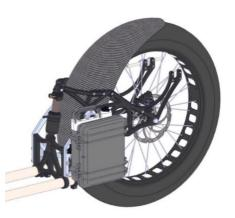
The battery is locked in place via a secure magnetic locking system under typical operating conditions.
