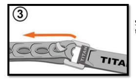
Stretch and secure the strap over flange. The tension in the strap is what secures it in place.
